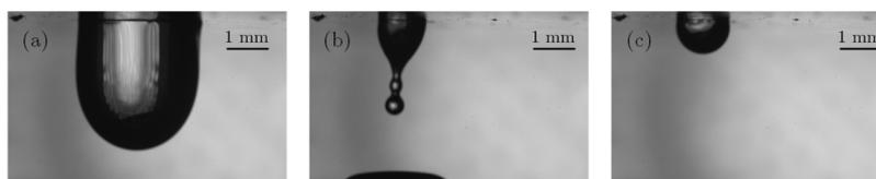
**Figure 12.** Example of a pendant droplet sustained by the electric field (a). After switching the electric field off, the droplet detaches from the surface (b), and a residual droplet sticks to the surface (c).
