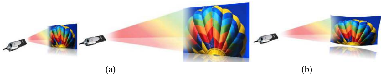
Figure 3. Unique properties of the pixel scanning based laser projector: (a) Stays focus when changing focal length; (b) Project on any shape surface
